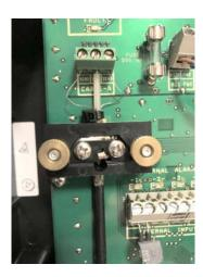
To remove the strain relief block (which is also the cable jacket stripping tool) from the circuit board, unscrew the two (2) outer brass thumb screws. The two smaller inner screws hold the stripper tool blade in place. **Do not loosen these screws.**
