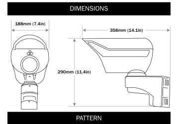
Model 420 provides a narrow, well-defined detection pattern with a maximum range of 122 m (400 ft) and a maximum width of 3.3 m (11 ft). The detection pattern is actually comprised of two fields-of-view that establish a narrow curtain of coverage in the area to be protected. Vertical detection pattern is approximately 26 degrees, measured downward from the detector axis. Typical horizontal and vertical detection patterns are shown below.
