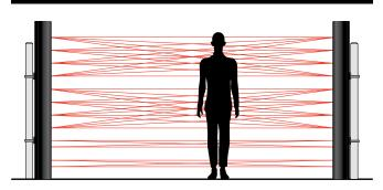
Intrusion alarm is triggered when at least one beam set is broken between transmitter and receiver. A time-delay triggered alarm is generated when one beam is broken.
