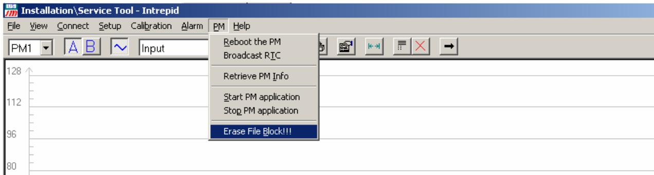
In the event of data corruption it is necessary to perform the above keystrokes during start-up of the PM's application software. To accomplish this, remove power from the PM board by unplugging one of the PCC cables located at the front of the PM board. Upon reapplication of power the PM will begin boot-up. During boot-up repeat the keystrokes as many times as possible.
