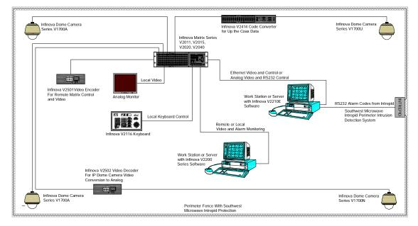
Also displayed in the diagram are associated Infinova control system options, such as, UP the COAX code converter (V2114), IP Video Decoder (V2502) for conversion of the V1700N series Infinova IP Dome video bit stream to analog video, and the IP Video Encoder (V2501) for remote Matrix control and video using the Infinova V2000 series software
