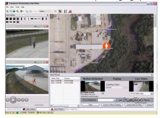
Unlike, less capable systems, PureActiv continues to control the PTZ camera to follow the target, even when it moves out of the field of view of fixed cameras. As the target moves, in addition to controlling pan and tilt, PureActiv controls the zoom to keep an optimal view of the target throughout the following process.
